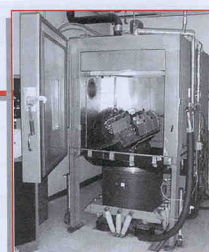
FIG. 4-A—Chamber/shaker for ESS using a skewed table on an electromagnetic shaker.
